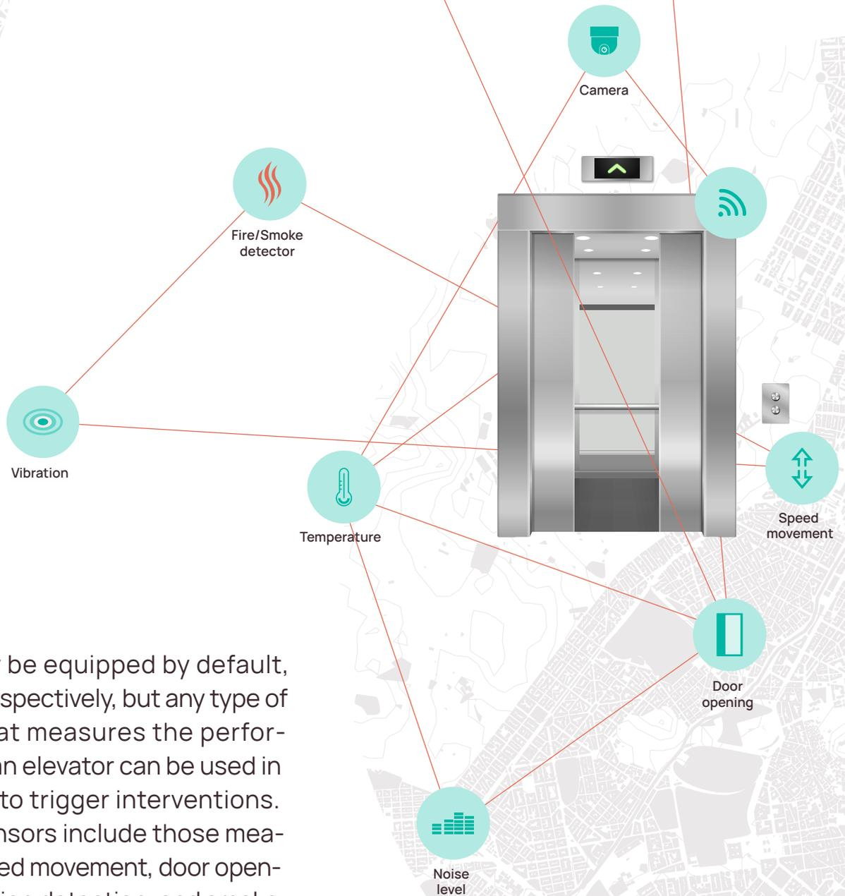
Some may be equipped by default, other retrospectively, but any type of sensor that measures the performance of an elevator can be used in Fieldcode to trigger interventions. Typical sensors include those measuring speed movement, door openings, vibration detection, and smoke detection.
